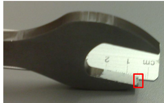
Figure 7.10: The contact surface for the lower jaw is 0.5 mm from the outer edge.
